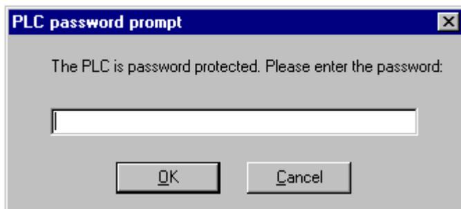
If you enter the correct password and confirm the dialog with <OK>, the login to the PLC is performed.
