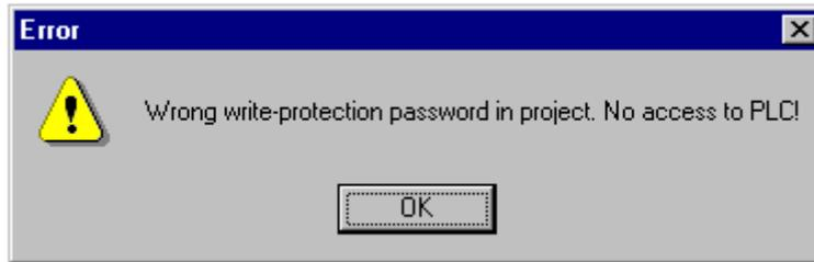
After you confirm this message with <OK>, another message appears displaying which project is loaded on the controller. Then the login is aborted.
