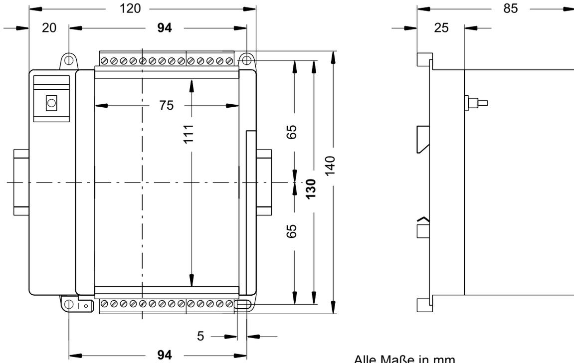
**The device is 85 mm deep.** If a DIN rail is used, the mounting depth is increased by the overall depth of the rail.
