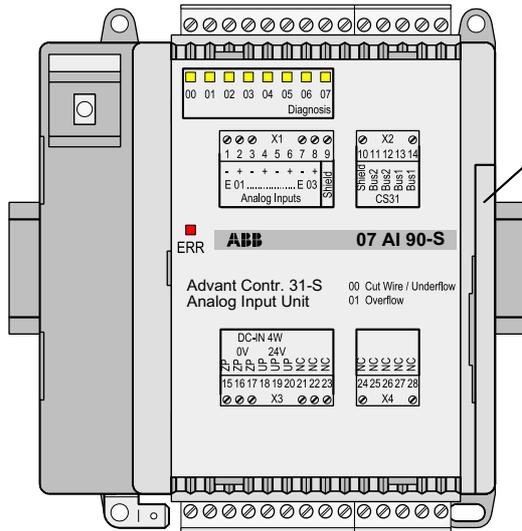
Setting the module address (0...5) is done using a DIL switch. The switch is accessible after removing the lateral cover. Pull the cover towards the front while tilting it lightly to the right. The switch is provided with a lid.
