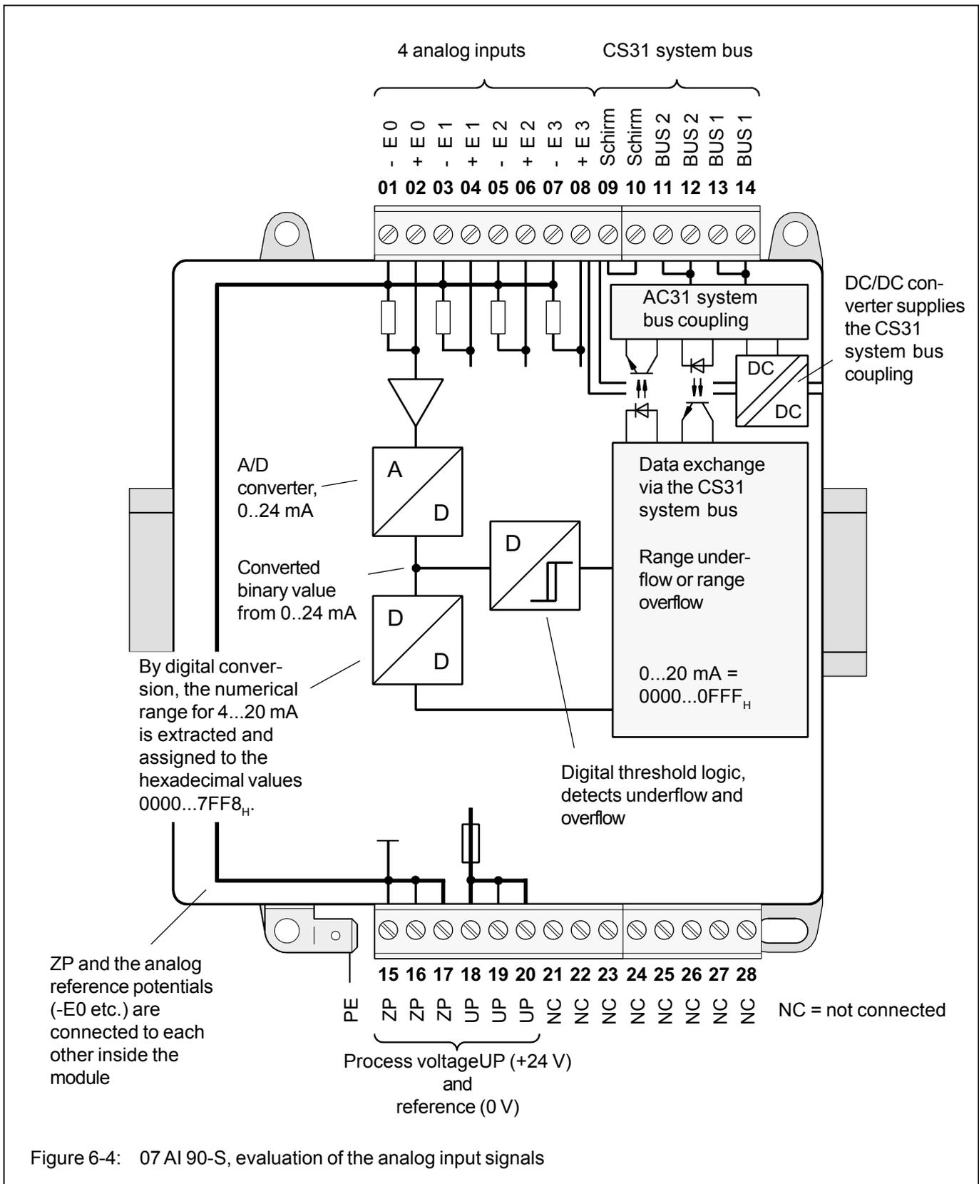
Figure 6-4: 07 AI 90-S, evaluation of the analog input signals
